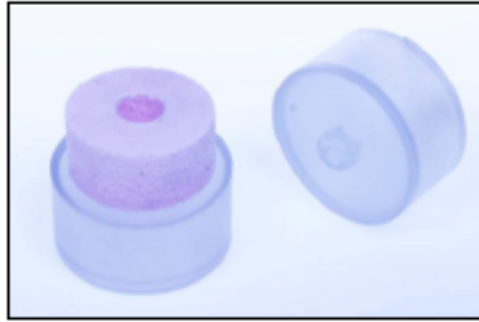
Figure 2: The micro CT cold stage. Dry ice is loaded in the top and bottom hollow containers and the specimen is placed in the center region.
